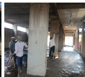
NDT by rebound hammer test at Restaurant construction site, Muddebihal by Prof. R. H. Baragani
