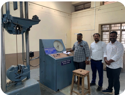
Tensile strength of HYSD Steel bar using Universal Testing Machine
