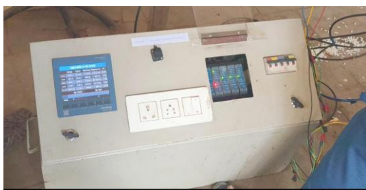
Fig(1&2)Power analyser : measures the voltage current real power reactive power powerfactor harmonics of R Y B and neutral and 2-phase line ... it consist of ct probes that are used for non-destructive measurement
