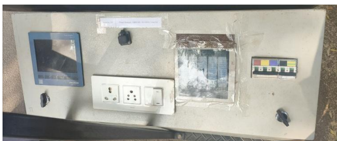
Fig(1&2)Power analyser : measures the voltage current real power reactive power powerfactor harmonics of R Y B and neutral and 2-phase line ... it consist of ct probes that are used for non-destructive measurement
